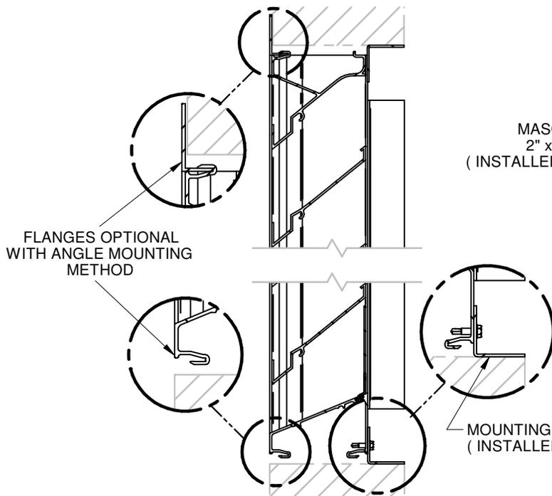
**METHOD D - MASONRY STRAP MOUNTING**
