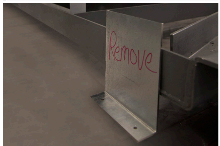
FIGURE 10: TYPICAL FAN BASE SHIPPING BRACKET ▼
