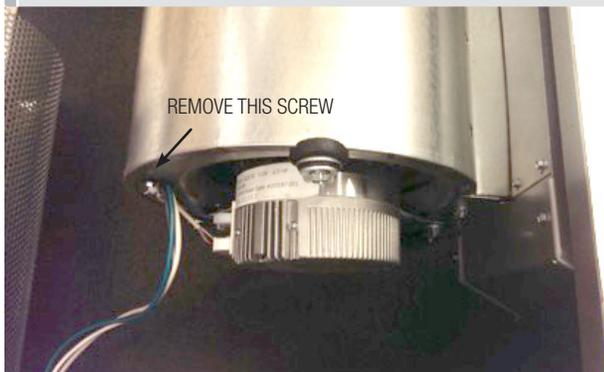
FIGURE 3: PSC MOTOR WIRING ▼
