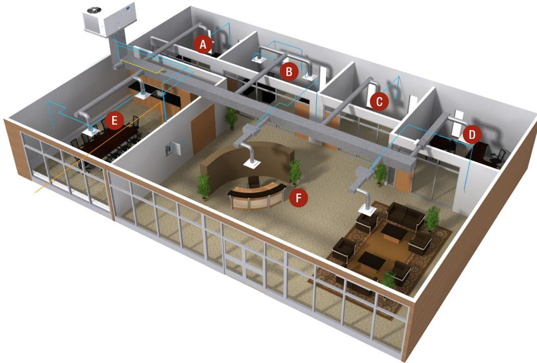
In an all air system, the supply air (typically provided at a fully saturated 55 degrees F) would provide the required cooling. The cool air requirement is typically much larger than the ventilation requirement, and varies with respect to the ventilation requirement for each zone ( $Z_{req}$ ).
