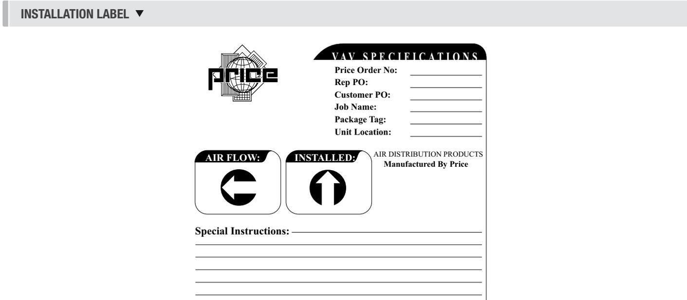
If there is a need to reposition the terminal unit to an orientation other than that indicated by the factory label, the following items must be considered prior to repositioning the unit.
