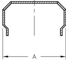
– TYPICAL RECOVERED SHAPE OF VINYL BLANK-OFF AFTER INSTALLATION.
