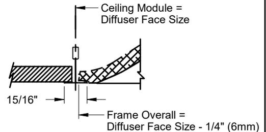
ALL METRIC DIMENSIONS ( ) ARE SOFT CONVERTED. IMPERIAL DIMENSIONS ARE CONVERTED TO METRIC AND ROUNDED TO THE NEAREST MILLIMETER.
