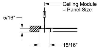
17P - 9/16" Bolt Slot T-bar
